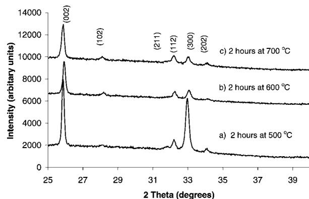
Figure 3 XRD traces of thin film pure HA, annealed for 2 h at: (a) 500 °C, (b) 600 °C, and (c) 700 °C.
