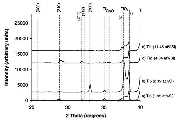
Figure 4 XRD traces of thin film SiHA on titanium substrates, annealed for 3 h at 600 °C: (a) Ti5, (b) Ti1, and (c) Ti7, (d) Ti2 (see Table I).
