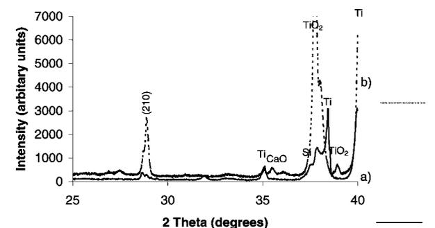
Figure 5 Effect of heat-treatment time on texture and crystallinity of thin film Si-HA on titanium substrates: (a) Ti7 heat-treated for 3 h at 600 °C and (b) Ti7 heat-treated for 24 h at 600 °C.
