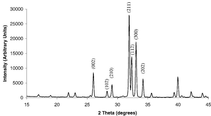
Figure 2 XRD trace showing phase purity of the HA target material.
