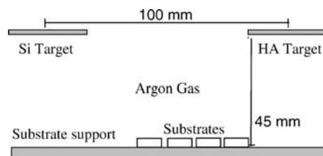
Figure 1 Setup for thin film SiHA sputter deposition.
