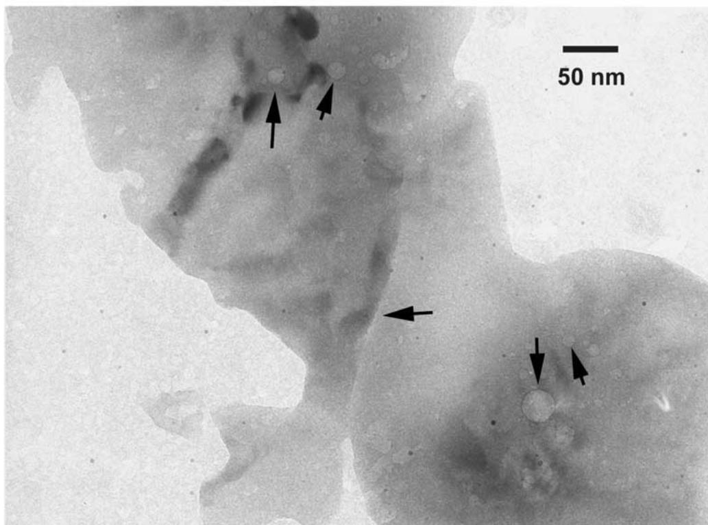
Figure 6 (a) TEM micrograph of SiHA crystallites. (b) TEM micrograph of SiHA illustrating the presence of grain boundaries and voids.
